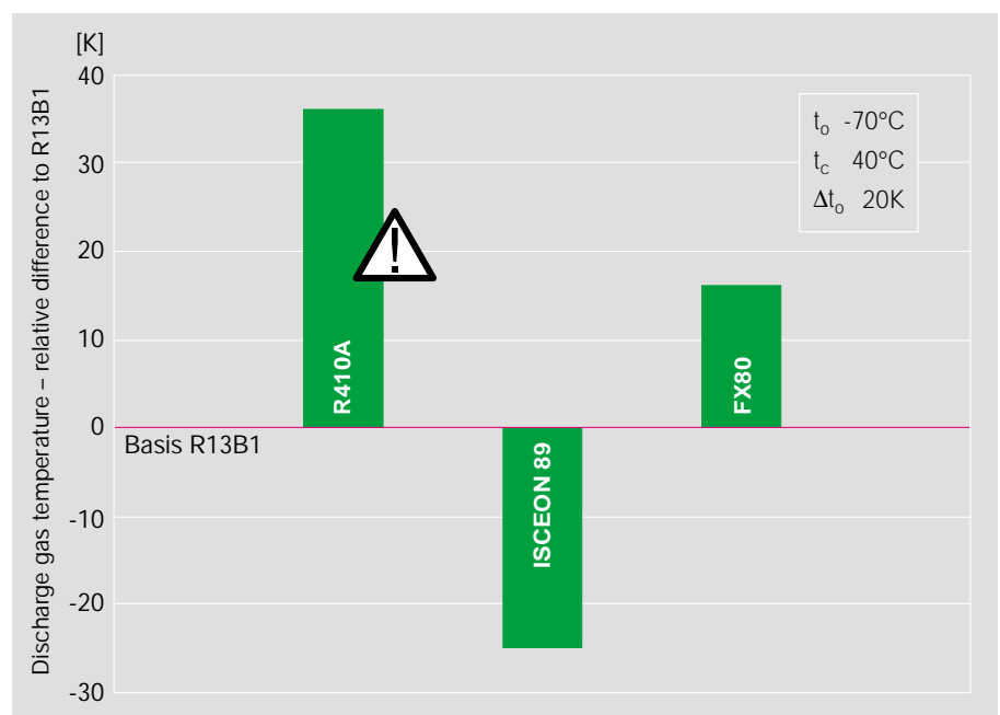
Abb. 31 R13B1/HFC alternatives – Comparison of discharge gas temperatures of a 2-stage compressor
